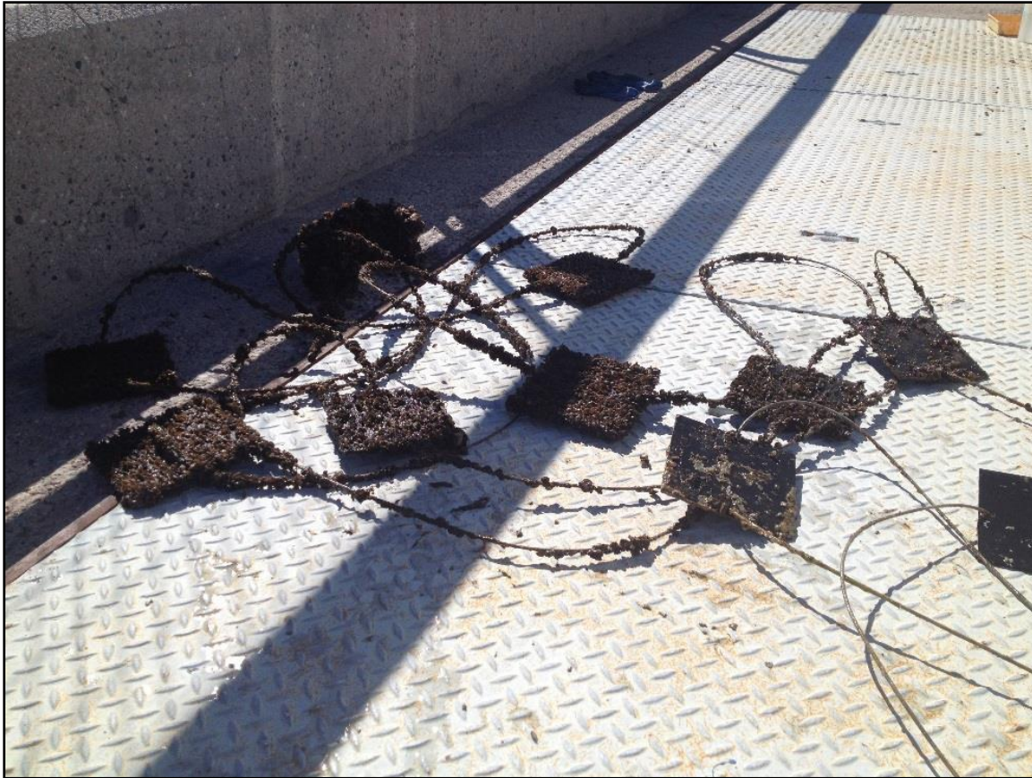
Figure E3. An example of a stringer of settlement monitoring plates heavily colonized by quagga mussels.
