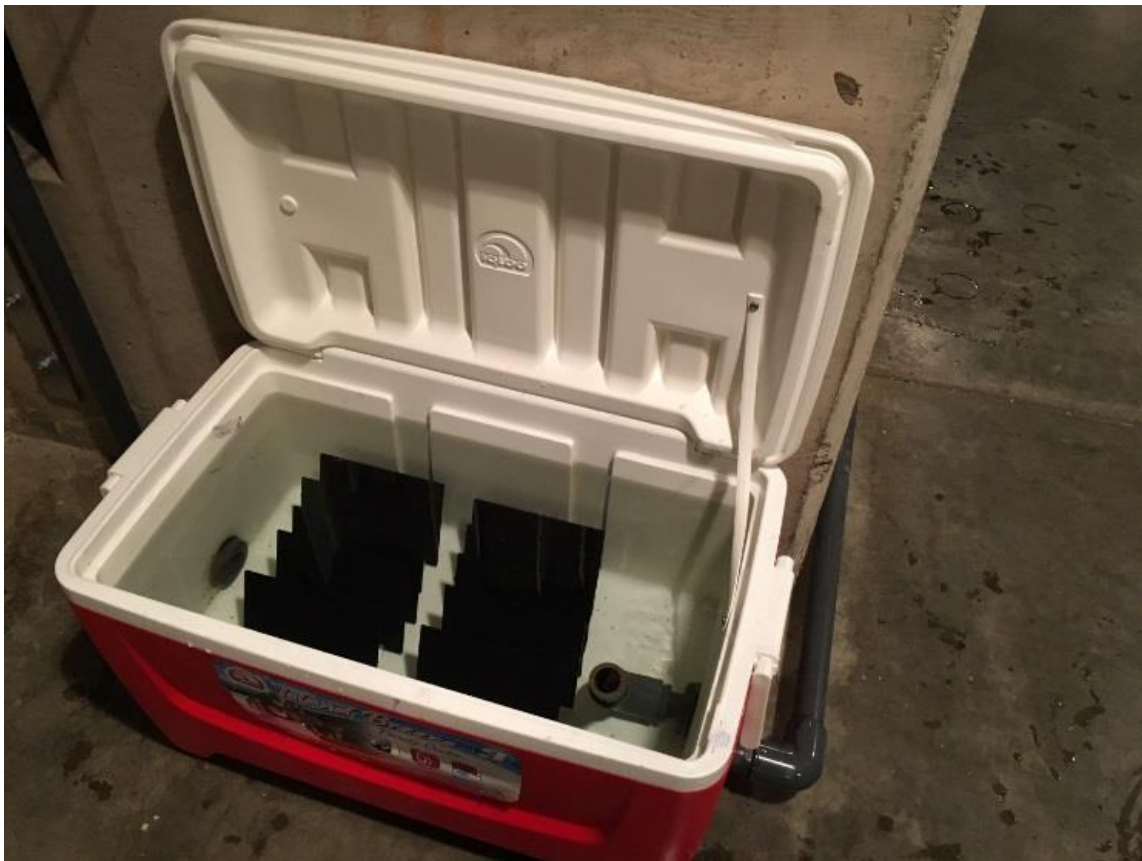
Figure E-4. Example of a biobox setup in a modified cooler with mussel settlement substrates.
