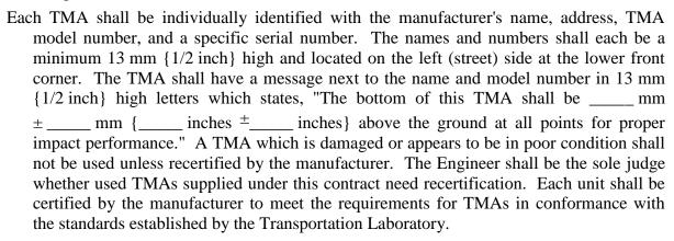
Approvals for new TMA designs proposed as equal to the above approved models shall be in conformance with the procedures (including crash testing) established by the Transportation Laboratory. For information regarding submittal of new designs for evaluation contact: Transportation Laboratory, 5900 Folsom Boulevard, Sacramento, CA 95819.
