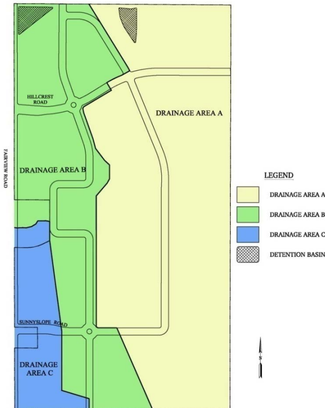
FIGURE 6-1 STORM DRAINAGE AREAS
