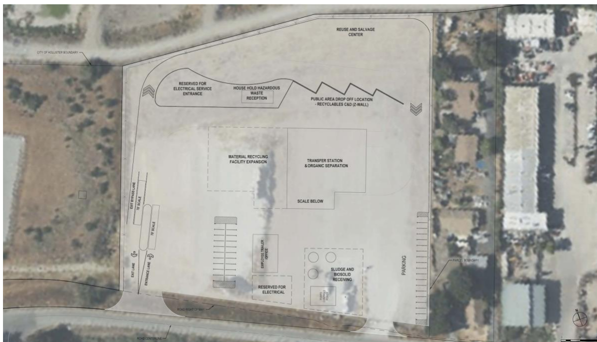
Figure 1: Conceptual Layout of the new Waste Transfer Station
